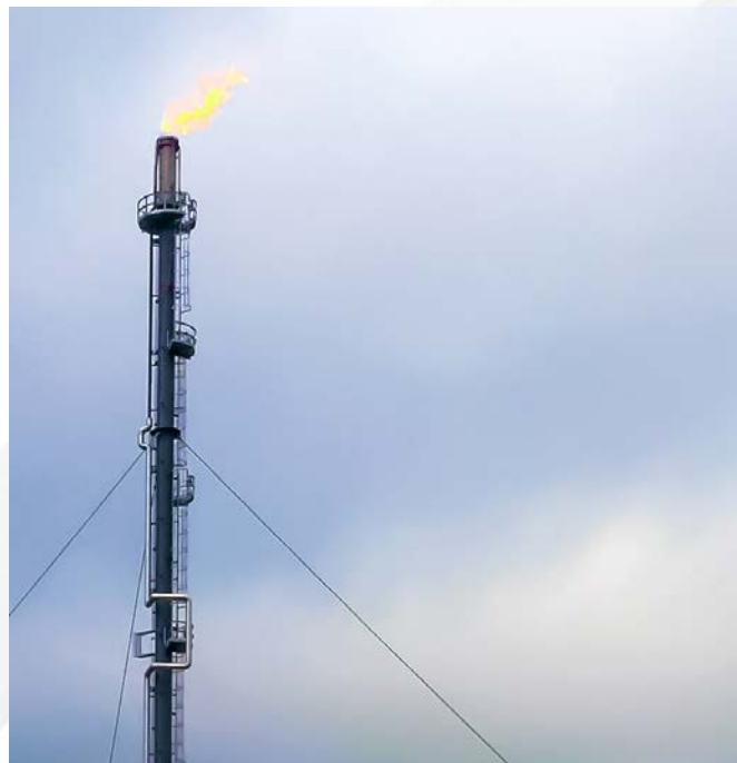
Proper application of steam allowing luminosity in the flame and full combustion
