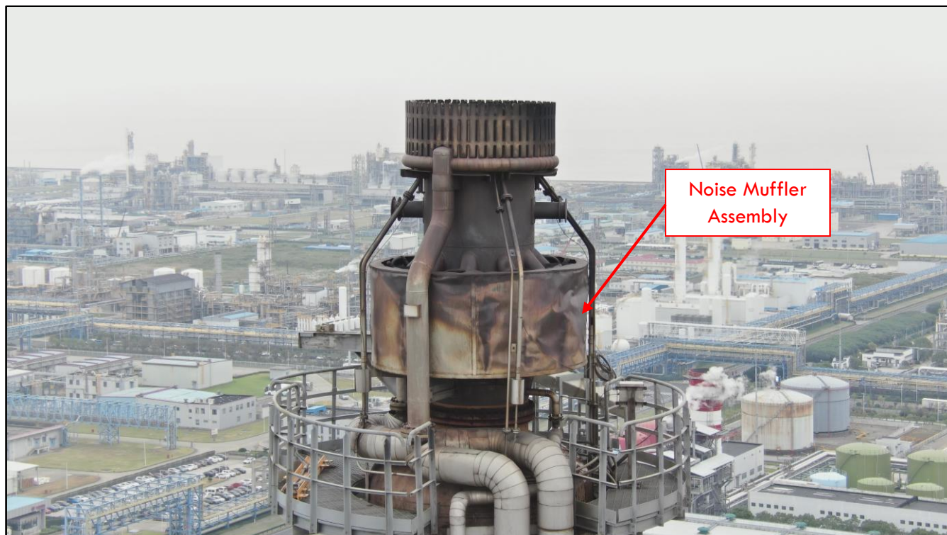
FIGURE 08 – Internal burning has occurred in the noise muffler due to flashback in the steam tubes. This indicates breakage in steam tubing, and a lack of continuous steam flow. Continuous flow is required through steam injection components to provide cooling and prevent flashback. Ensure continuous cooling steam is run to the flare tip per manufacturer recommendations.
