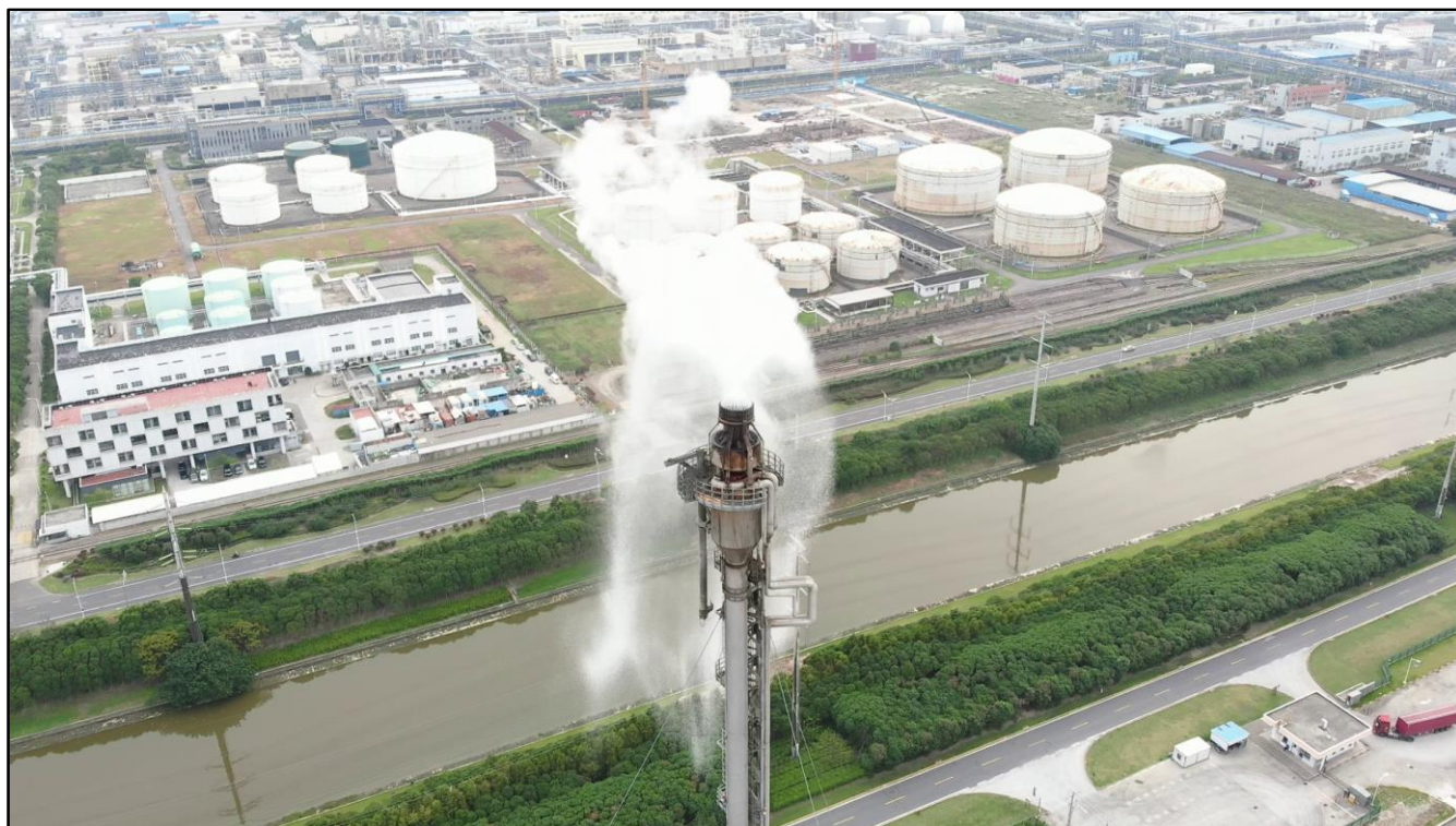
FIGURE 10 – When steam rate was increased, a significant amount of water exited the steam injectors. Zeeco recommends improving steam quality to improve smokeless performance and extend the lifetime of steam injection components. Another option to consider is heat tracing steam risers.
