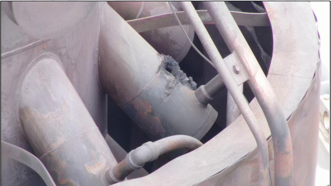
FIGURE 05 – A hole was detected in the steam tubes. Smokeless capacity has been compromised.
