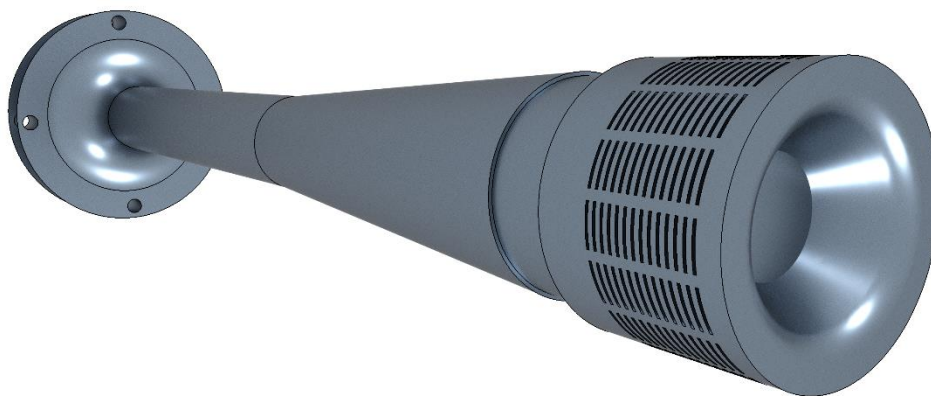
Figure 6. Simulation geometry of the venturi with horizontal slot RWSF burner.
