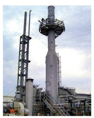
ZEECO Vertical Tank Vapor Thermal Oxidizer
