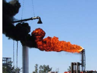
Visible Image of Smoking Flare
