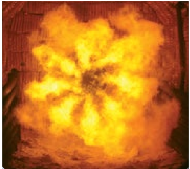
ZEECO GB Low-NO x Power Burner
