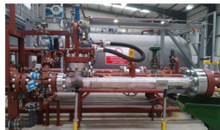
Figure 12. Photo of FAT Test of Liquid Ejector
