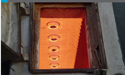
Fig 2: GLSF downfired burners firing with mixed fuel gas
