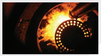
ZEECO<sup>®</sup> thermal oxidizers reliably and safely destroy BTEX and amine acid gas streams with 99.999% DRE
