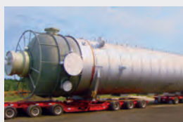
Tail Gas Thermal Oxidizer designed and built to GOST-R requirements. Zeeco can meet local standards throughout the world such as GOST, CE, CSA, etc.
