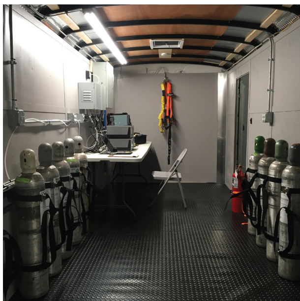
Figure 3. Mobile test laboratory equipped for RATA testing in the presence of methane.
