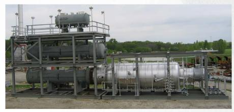
Modularized SRU Reaction Furnace
