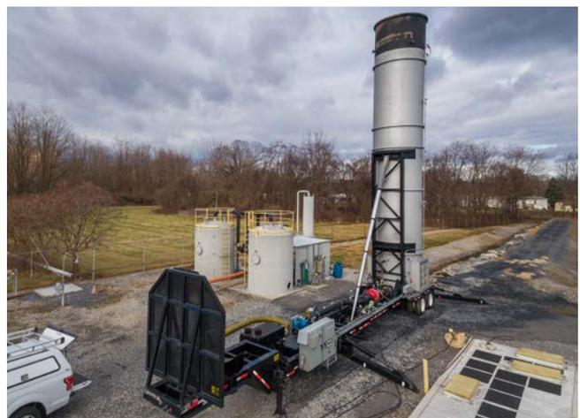
*Zeeco's Zephyr portable VCU*
