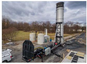
Zeeco's Zephyr portable VCU
